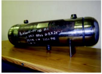
Fig. 2 — Portion of the root not welded and partial weld deposition of remaining head to shell joint.
