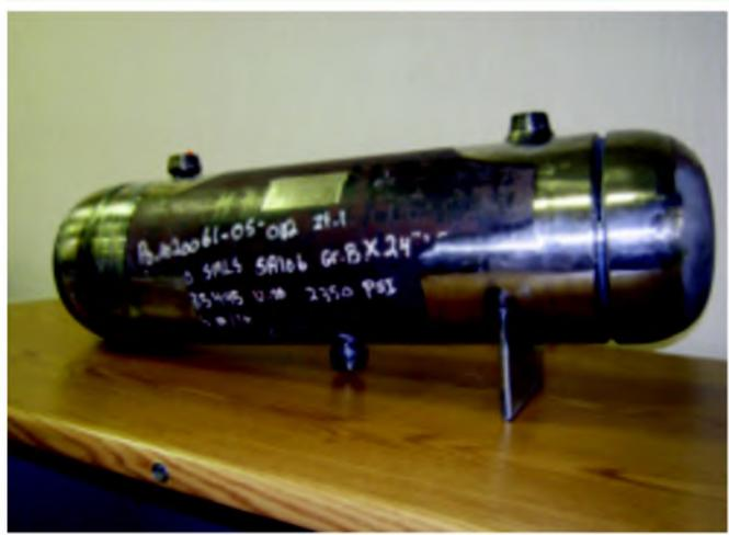
Fig. 2 — Portion of the root not welded and partial weld deposition of remaining head to shell joint.
